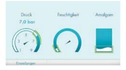
The 4,3" colour touch screen enables the monitoring directly at the Power Tower. Thanks to its network compatibility it can be monitored via the PC directly at the reception. All important parameters are constantly under control and should any failure take place they are reported immediately.
